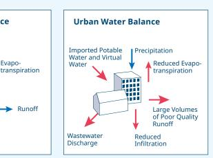
Fig. 18: Comparison of how a typical city and water-sensitive city affect the natural water balance
