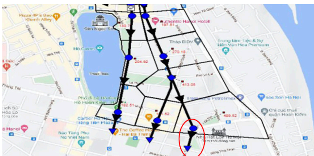
Figure 3: Delineation of the case study area in SWMM model: Delineation of catchment area based on the topology, the location of manholes and sewer network in SWMM model (red circle is the simulation note for calibration between observed and simulated flood event)
