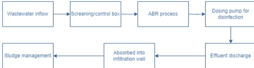
Figure G.2. Communal WWTP diagram
