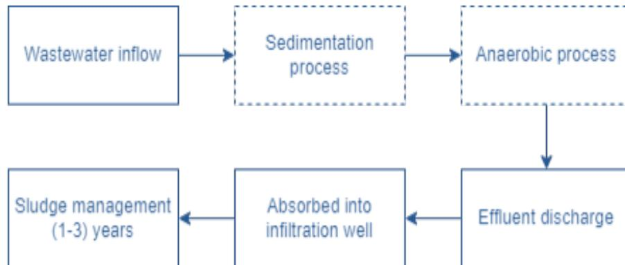
**Figure G.1. Improved septic tank diagram**
