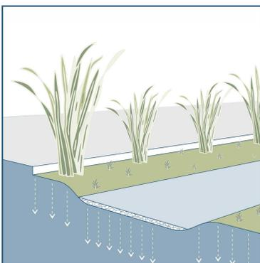
Excavated trenches filled with stones to create basins capable of retaining rainwater. This stored rainwater gradually seeps into the ground over a period of several days.
