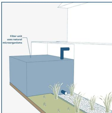
A wastewater treatment system utilizing natural microorganisms on a support medium to decompose pollutants, thereby restoring the water to a clean state.
