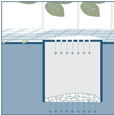
Well or pit in the ground into which flows rainwater drainage.
