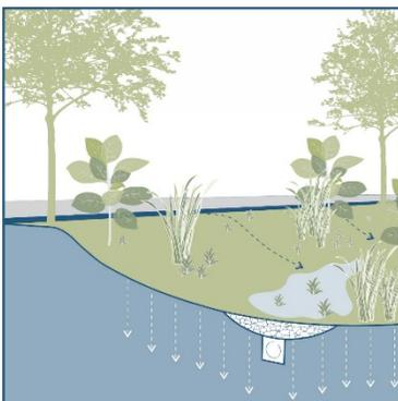
Shallow, flat bottomed, vegetated open channels designed to convey, treat and often attenuate surface water runoff.
