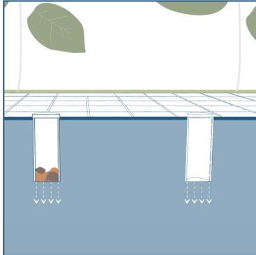
A hole with a diameter of 10-30 cm with a length of 30-100 cm which is covered with organic waste which functions to trap flowing water so that it can become a source of water reserves for underground water.
