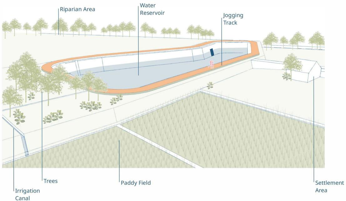
Build water reservoirs to ensure water availability for agricultural land and channel it through irrigation canals. Water reservoirs also function as rainwater catchment and help control floods
