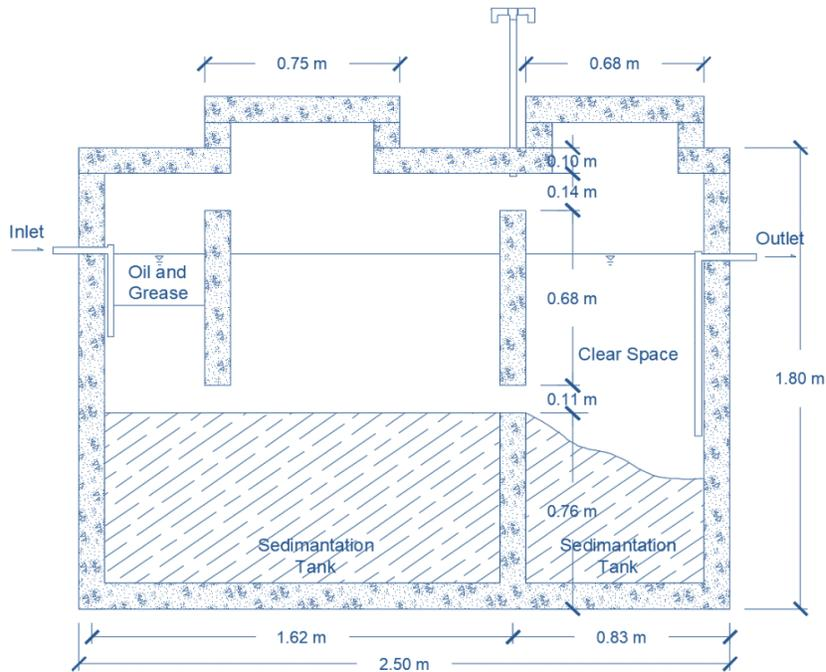
Figure G.5. Cross Section A-A' for Market WWTP
