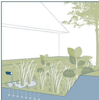
Constructed wetlands for phytoremediation uses the application of plant-based processes to improve hazardous contaminant conditions, aiming to obtain cleaner water.
