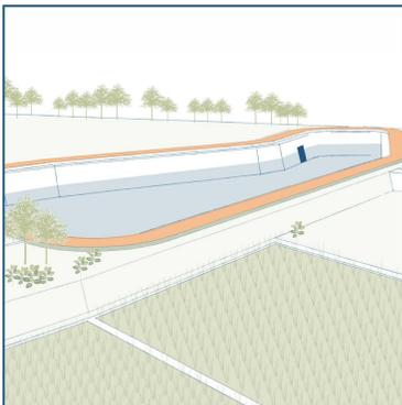
Ponds or pools designed with additional storage capacity to attenuate surface runoff during rainfall events and use the water during the dry season.
