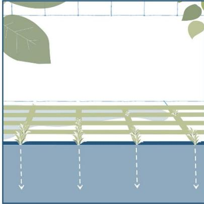
The construction material aims to augment infiltration areas, facilitating efficient water percolation into the soil, reducing inundation, and enhancing groundwater reserves.
