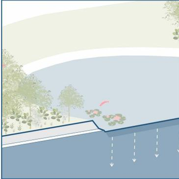
A strategically designed and landscaped depression or shallow basin that captures, absorbs, and filters stormwater runoff from roofs, driveways, sidewalks, and other impermeable surfaces.
